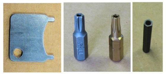
This tool is used for removal and refitting of spray nozzles only
