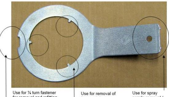
Use for ¼ turn fastener for removal and refitting of old-style soap dispenser lid (pre 2012) Use for removal of foot push button housing Use for spray nozzle removal / refitting
